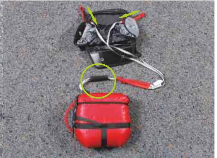
2. Fix the Y-bridle in the required position on the front container by using the velcro strips. Connect the parachute bridle with the Y-bridle of the front container (for details see No. 3)
