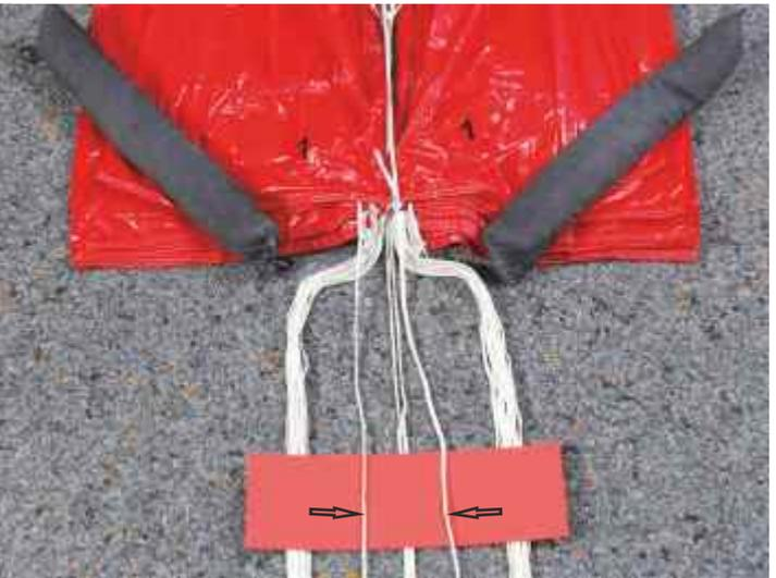
16. Check line 1 and 2 (arrows) and the center lines are not crossed and running free.
