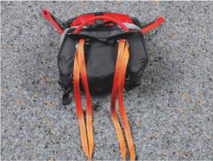
6. Close the bottom flap and secure provisionally with the pins of the release handle.
