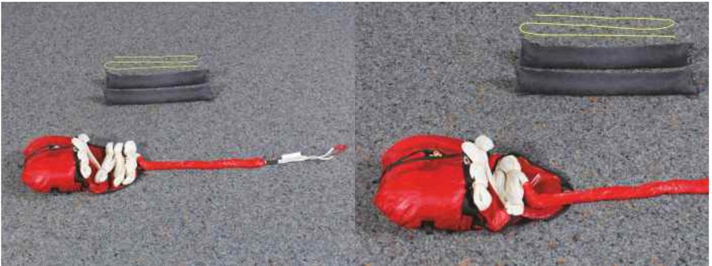
21. Close the canopy deployment bag with the lines. First in the middle then the sides. Bundle the lines in 3x3 "8-shaped" hanks. Do not bundle the last 60 cm of lines.
